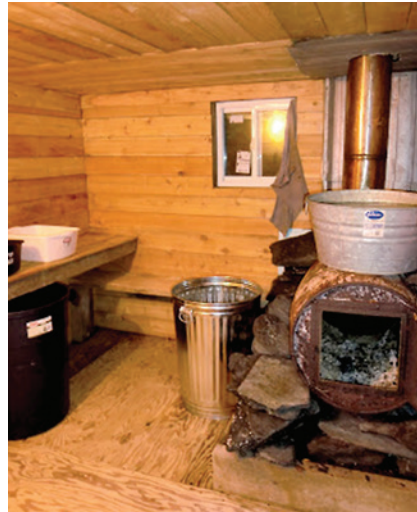
River stones around a 55-gallon drum wood stove, benches and a big pot of water. Traditional Russian baths include gentle beating of the skin with a grass or leafy bundle called a venik [below].
