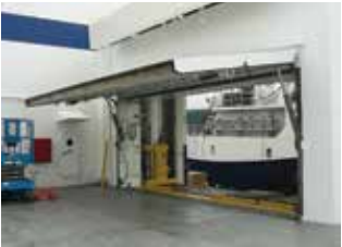
The unique elevator installed on the new M/V Coastal Standard allows the vessel to load and offload palletized frozen cargo quickly via forklift. Photo courtesy Dakota Creek Industries.
